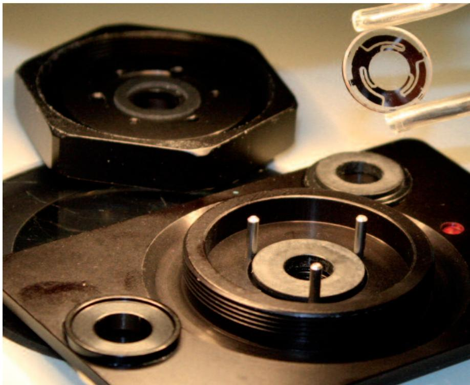
A lithographically patterned calcium fluoride window (13 mm diameter) being lowered into a micro compression cell. The window is part of a specialised sample chamber that enables living cells to be studied by infrared microspectroscopy.
