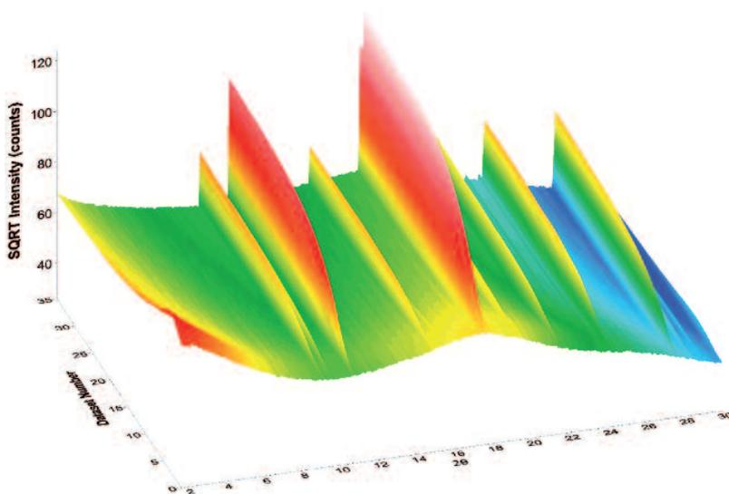
Accumulated synchrotron powder X-ray diffraction patterns showing the formation of jarosite from solution over time. The data are represented as a three-dimensional plot with diffraction angle ( $2\theta$ ) along the x-axis, dataset number (which relates to elapsed time) along the y-axis and intensity along the z-axis. The top figure views the data down the z-axis. The bottom figure views the patterns from an angle that clearly shows the growth of the jarosite peaks.
